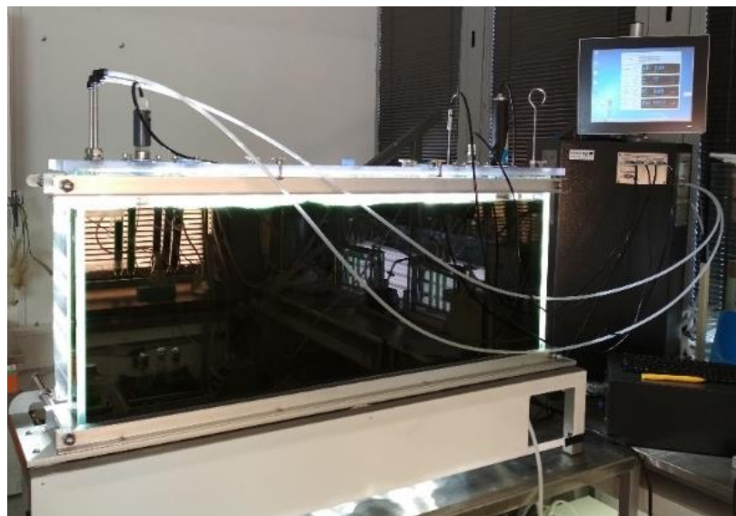
25-L flat panel photobioreactor
