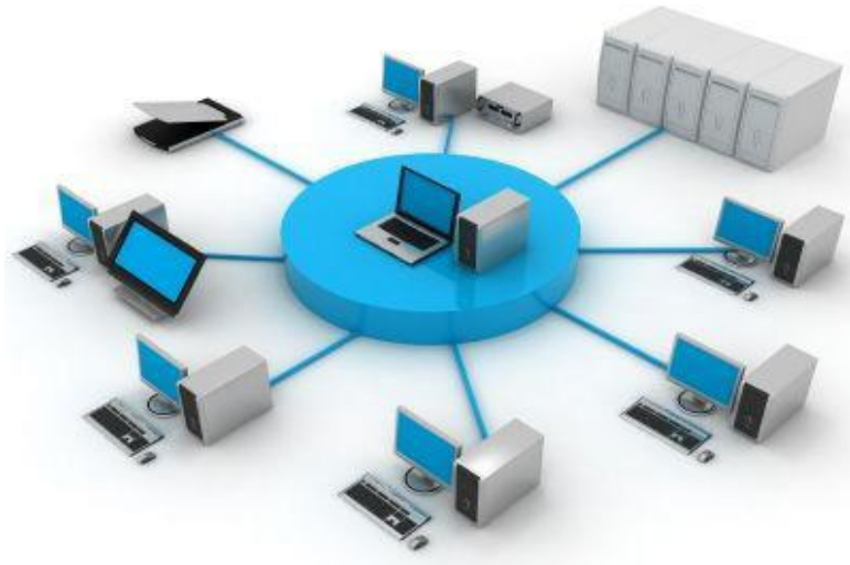
Picture 1: a star shaped network connection
