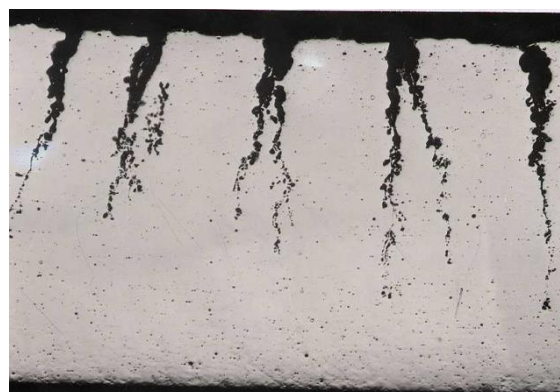
Figure 7.4 Microphotograph of corrosion cracking
