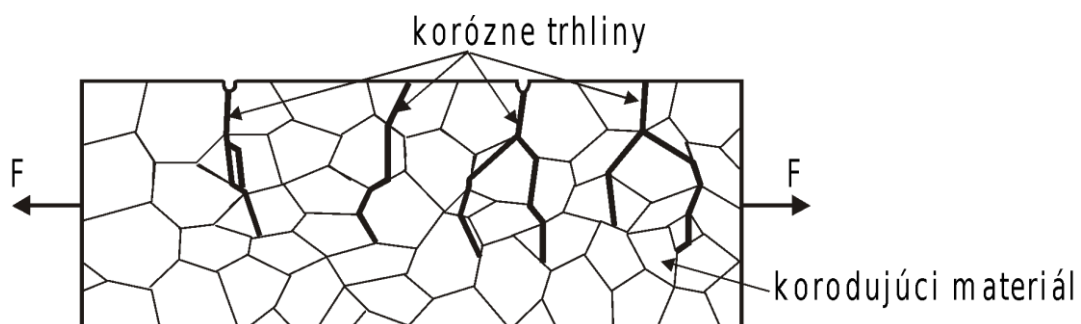
Figure 7.3 Corrosion cracking scheme
