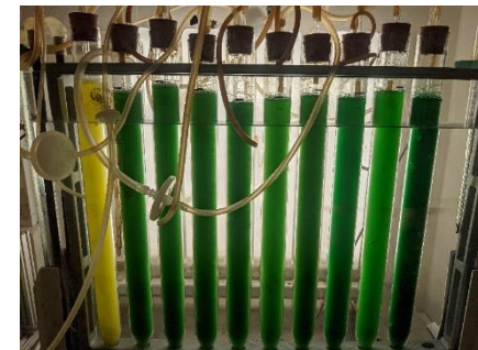
Fig 1 Cultivation in glass cylinders for the analysis of different types of wastewater.
