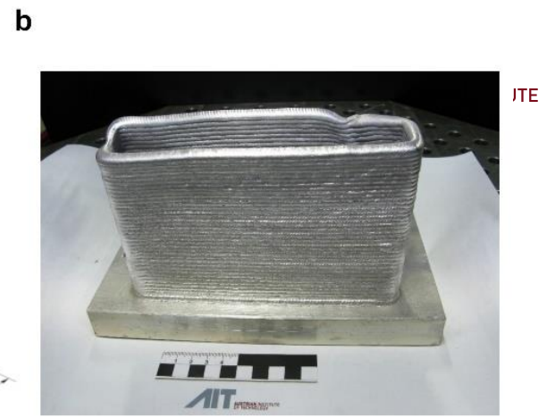
Details of the specimens fabricated for subsequent characterization. (a) Scheme inclusive tensile specimen locations; (b) photograph of the Mg AZ61A sample fabricated by WAAM
