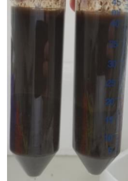
Energy crop digestate after centrifugation – dark colour remains even after dilution
