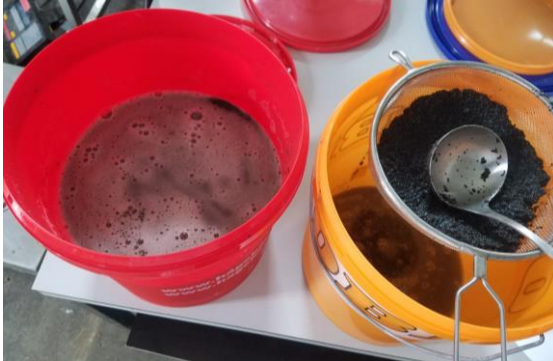
Sieving of dairy digestate Subsequent centrifugation necessary
