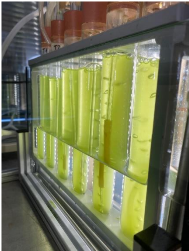
Fig. 4 Selection of best growing media for selected microalgae strains in 100mL cylinders.
