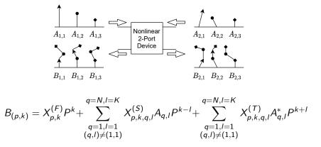
**Idea:** Apply a Large-Signal Tone at Port 1 and sweep an additional Small-Signal Tone with a slight frequency offset  $\Delta f$  for every Port and Harmonic  $\Rightarrow$  this leads to Lower and Upper Sidebands around the multiples of the fundamental frequency  $k \cdot f_0 \pm \Delta f$
