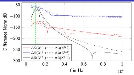
Since the common emitter amplifier is matched at 100 kHz and has the largest gain there, we also expect the largest X-parameters at this point and thus probably also high deviations from the AWR model
