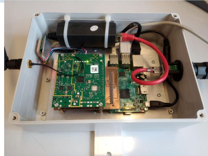
Test Setup with an iC880A
